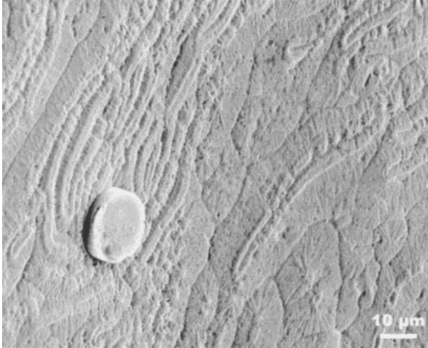
Figure 8 SEM micrographs of a specimen crystallized at 106°C for 10 min, showing row structures in a region where the melt was stretched.
